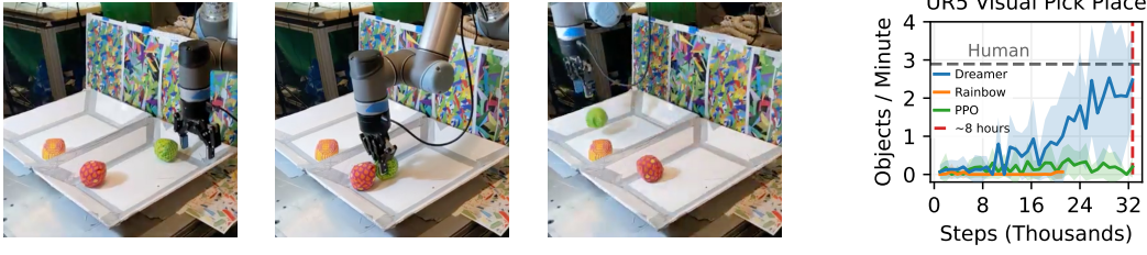
Figure 5: UR5 Multi Object Visual Pick and Place This task requires learning to locate three ball objects from third-person camera images, grasp them, and move them into the other bin. The arm is free to move within and above the bins and sparse rewards are given for grasping a ball and for dropping it in the opposite bin. The environment requires the world model to learn multi-object dynamics in the real world and the sparse reward structure poses a challenge for policy optimization. Dreamer overcomes the challenges of visual localization and sparse rewards on this task, learning a successful strategy within a few hours of autonomous operation.
