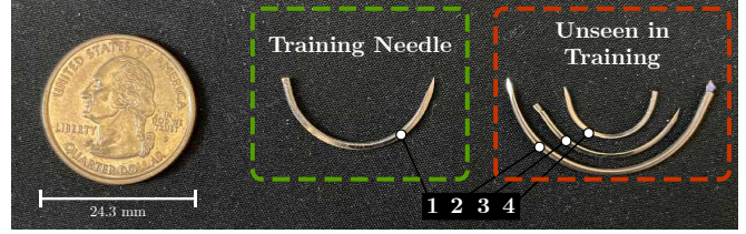
Fig. 7: Needles used: The needles are shown with a coin for scale. All models were trained using needle 1, while needles 2, 3 and 4 were also used for testing. Needles 1 and 3 have a radius of 1.25cm, and needles 2 and 4 have radii of 1.75cm and 0.75cm
