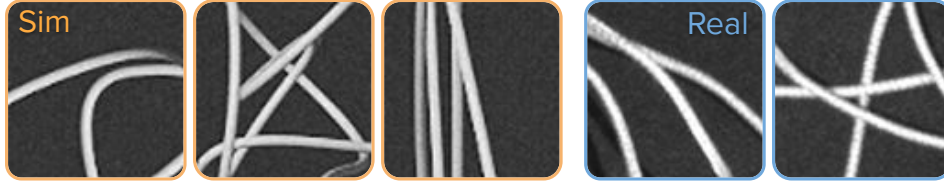
Figure 2: Cropped images of simulated and real cables for training HANDLOOM: On the left are simulated cable crops augmented with Gaussian noise, brightness, and sharpening to match the real images (right).
