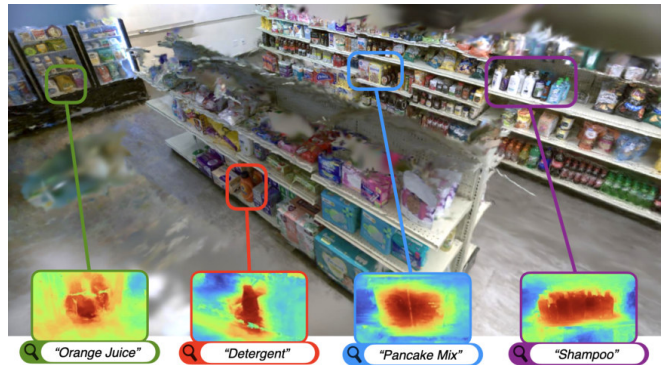
Fig. 1: Language-Embedded Gaussian Splat in TRI Grocery Store Testbed [15]. LEGS relies entirely on pretrained VLMs and does not require any inventory data or finetuning.
