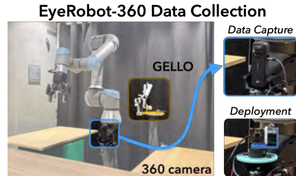
Figure 5: Teleop Data Setup with EyeRobot . We collect actions with GELLO [60], and the EyeGym environment with a time-synced 360 camera.
