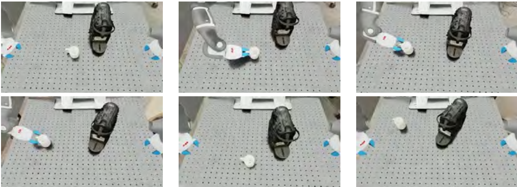
Figure 26: Random Lighting Augmentation Turned Off (Top Camera Views Shown). We turn off the randomized sphere light sources with varying colors and intensities. Uniform lighting is available from the only light source in the render scene – the skybox/dome-light asset.
