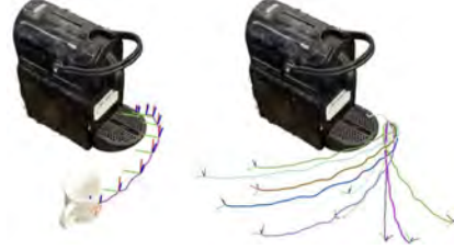
Figure 4: Trajectory Interpolation – R2R2R adapts object motion to varied start/end configurations via spatial normalization and Slerp.
