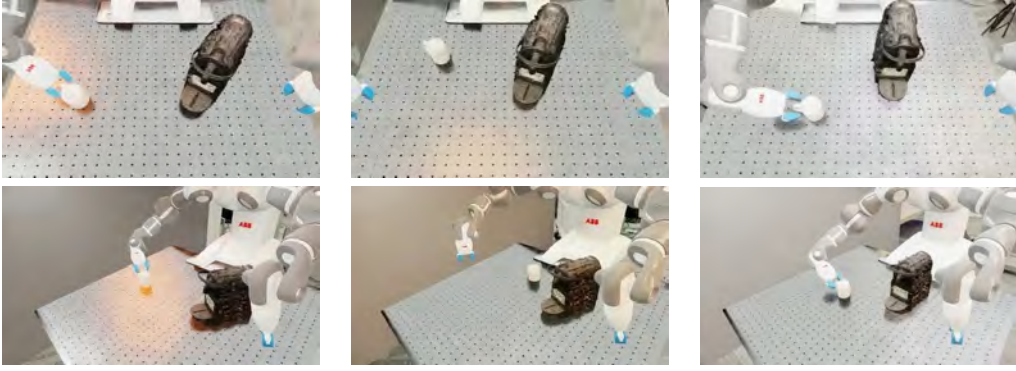
Figure 24: Real2Render2Real (Views From Both Cameras Shown). Base augmentations used in the main R2R2R experiments include: random sphere lighting, camera pose perturbation, robot initial joint perturbation, and randomized object initialization uniformly distributed via manual parameters.
