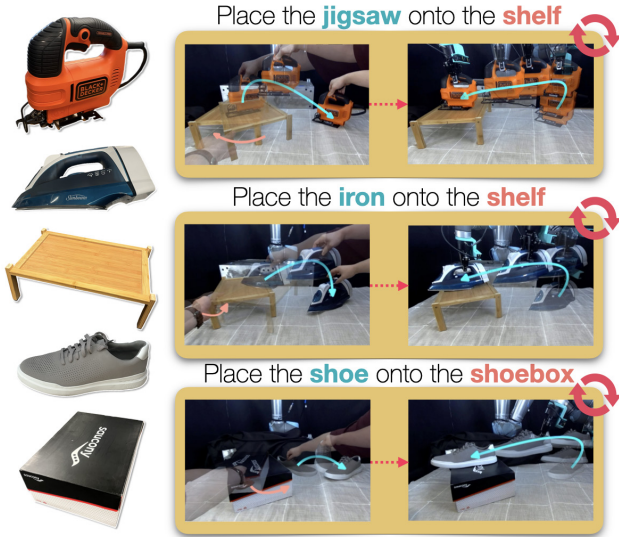
Fig. 4: Object Reset Experimental Setup Middle : A human randomly perturbs the configuration of the tracked objects according to the two tiers. Right : A robot arm then plans a grasp on language-queried objects and performs object reset. This process repeats until errors in object state estimation are too high to recover for grasping.
